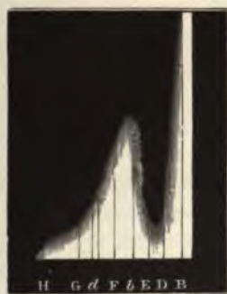
FIG. 80.—Absorption of various thicknesses of a solution of potassic permanganate. (Gladstone.)
